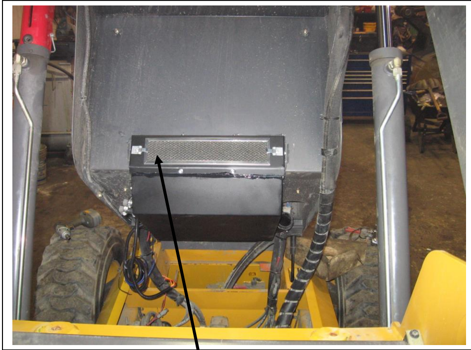
Install outside air filter cover and filter.
