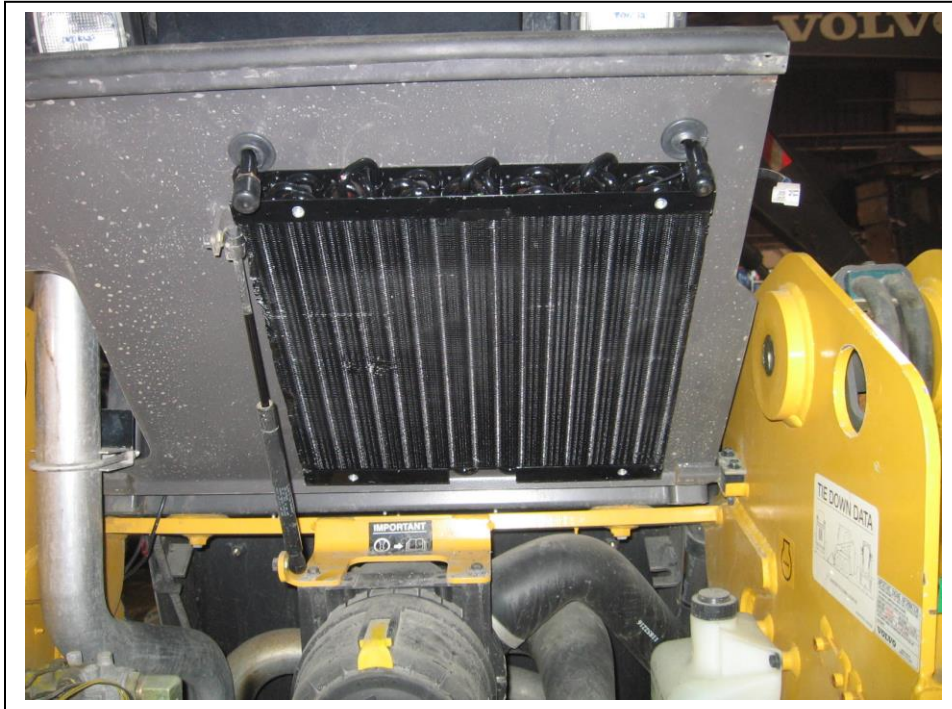
Coil fastens from top down. Bolt through the shroud, lid and into the coil.
